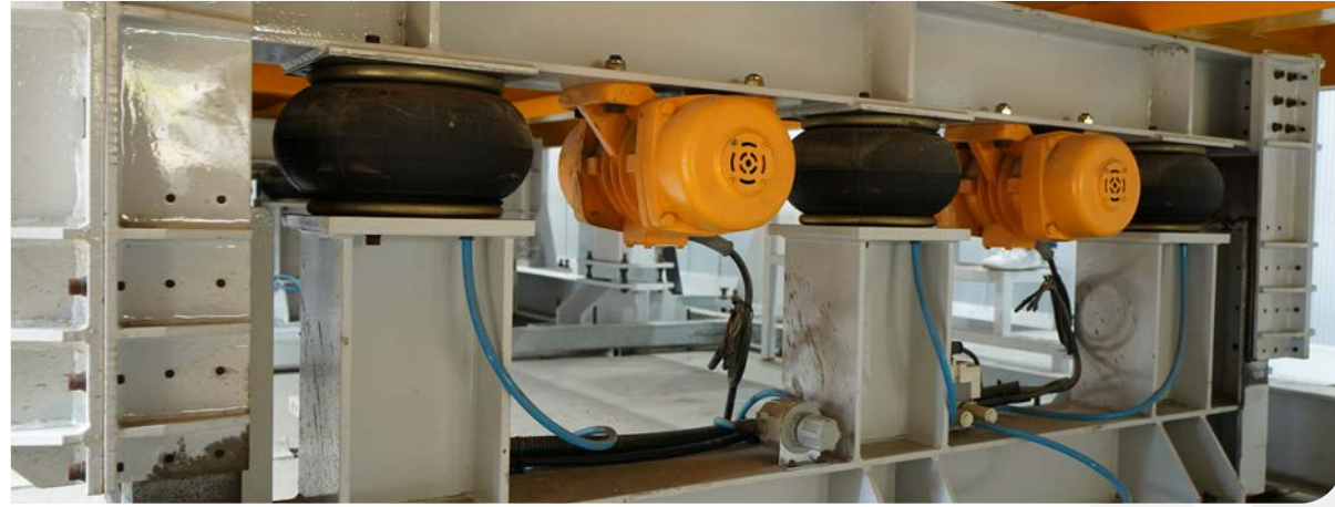
Step 7 Vibrator compaction
