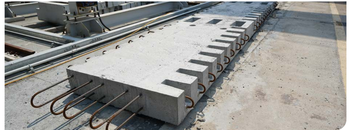
Step 12 Demolding and product transfer
