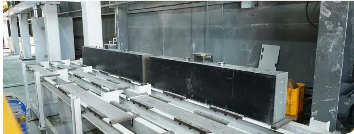
Step 2 Mold loading (using RFID)
