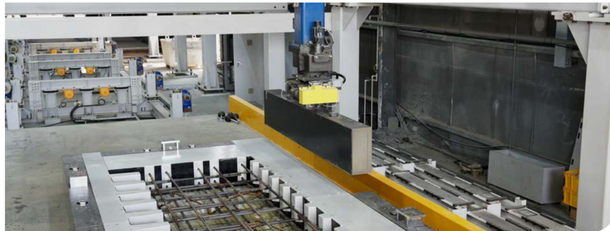
Step 3 Move mold to gripper
